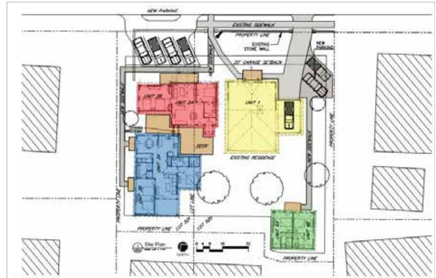
Figure 3-59. Example of an **inappropriate** site plan on E. Travis Street that proposes lot coverage far denser than the surrounding neighborhood. Note the contrast in setbacks between the proposed buildings and the surrounding historic buildings. Note also the proposed inappropriate parking location on the main street, with no buffering or landscaping. Source: City of Fredericksburg Historic Preservation Office.
