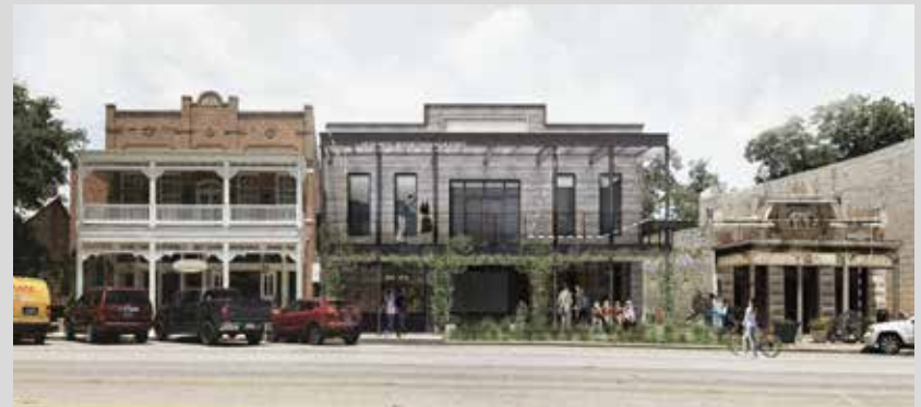
Rendering of the appropriate proposed new Albert Hotel on Main Street, designed by Clayton Little Architects. The new building shown at the center is compatible with its neighbors in terms of height, roof form, footprint, and the stylistic detailing of the parapet, but differentiated by its color, materials, and fenestration pattern. Also note the consistent setbacks and inclusion of a canopy. Source: Clayton Korte Architects.
